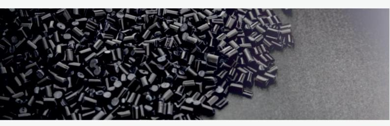
We Manufacture Black MBs in PE Base ranging from 35 % to 55 % carbon loading. The Carbon used are the best grade made from Tar and Oils. This gives high jetness and proper dispersion to the end product. Several additives are also added to give additional gloss to the Master Batch. Our Black MBs are compatible to use in HDPE Pipes, Injection Molding, Blow Molding, Films, etc. We also make Black MB in ABS, HIPS, PET, PS,PC and other such polymer Base.
